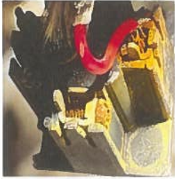
Picture is how device PT-02 was found. I reterminated wires, verified manufactures wiring diagram, tested and ok.
